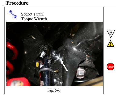
(i) Use a 15mm socket on the top bolt on the reinforcement bracket and torque to 60 N•m (Fig. 5-6).
