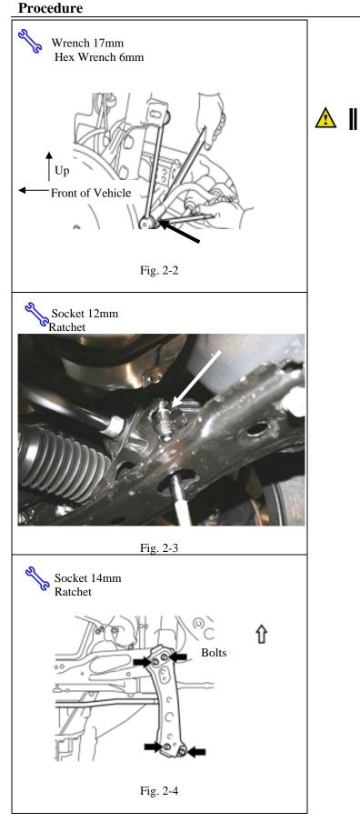
(b) Using a 17mm wrench and 6mm hex wrench, remove the lower nut (black arrow) on the sway bar end links on the RH and the LH side of vehicle and discard (Fig. 2-2).
